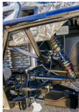
Double a-arm suspension is found front and rear, and the shocks are three-way adjustable.
