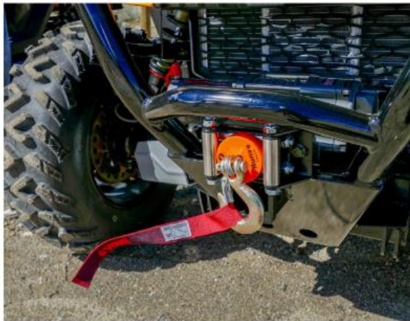
A great standard accessory on these Challenger models is a 3500lb winch.
