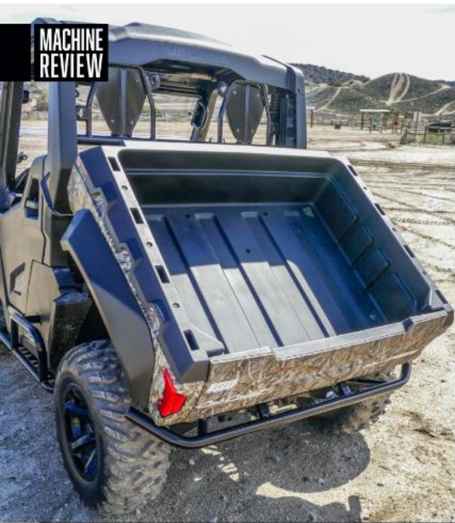
A standard dump bed can be actuated from both sides of the vehicle.
